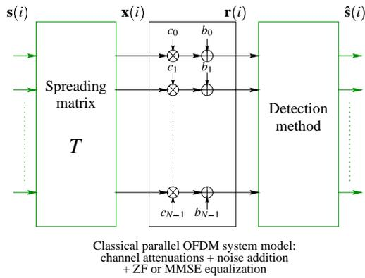
Fig. 1. Classical frequency domain SOFDM transmitter
